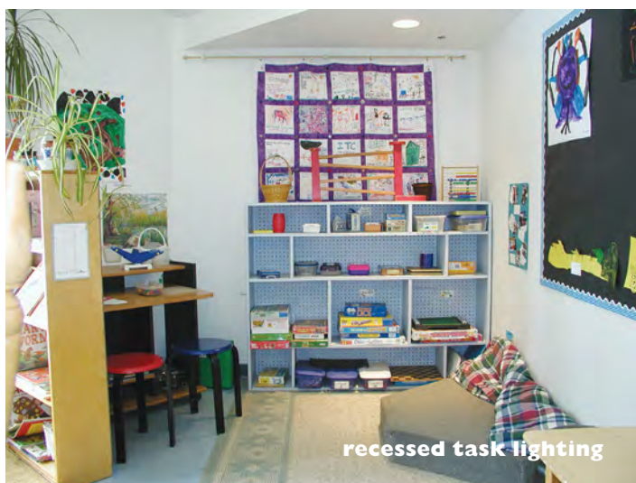
ABOVE: This center uses recessed task lighting to provide direct lighting for an activity area and further define and separate that part of the classroom. Notice the pool of light on the floor that marks the center of the area and will become the natural focus of activity.
